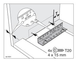
Screw the brackets onto the right and left inside walls of the housing unit as shown. The back edge of the brackets should align with the vertical line drawn up from the front of the spacer strip, and the lower edge aligned with the lower edge of the housing unit side wall. The brackets are designed for 16
